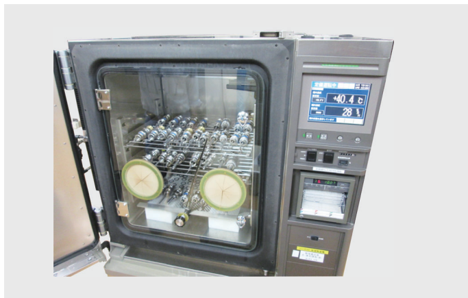
熱安定性試験（恒温槽）外観 Thermal Endurance Test (Constant Temperature Chamber) - External View
